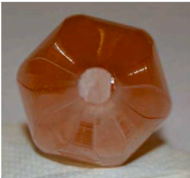
Fig. 6. Facets of LGT crystal ( \varphi \approx 50 mm) grown under stationary stable regime along Z-axis.
